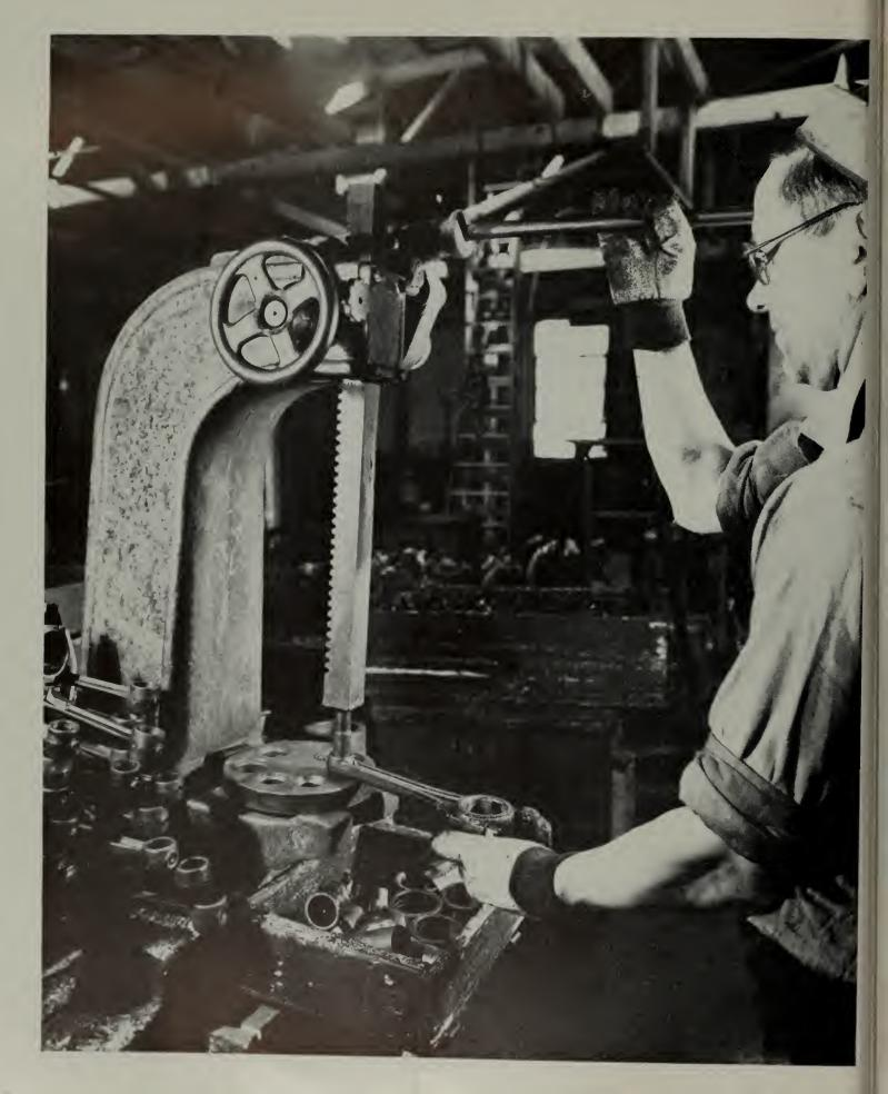
Other pin bushings have a heavy wall and are removed by use of an ordinary arbor press as shown above. It is much simpler and faster to remove the bushings in this manner.
